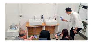
To visually illustrate the actual water savings, two aquariums were installed allowing the customers to check and measure the water consumption during the test in real time. The difference in the water levels between the two aquariums, evidently revealed the striking differences between the two products.
